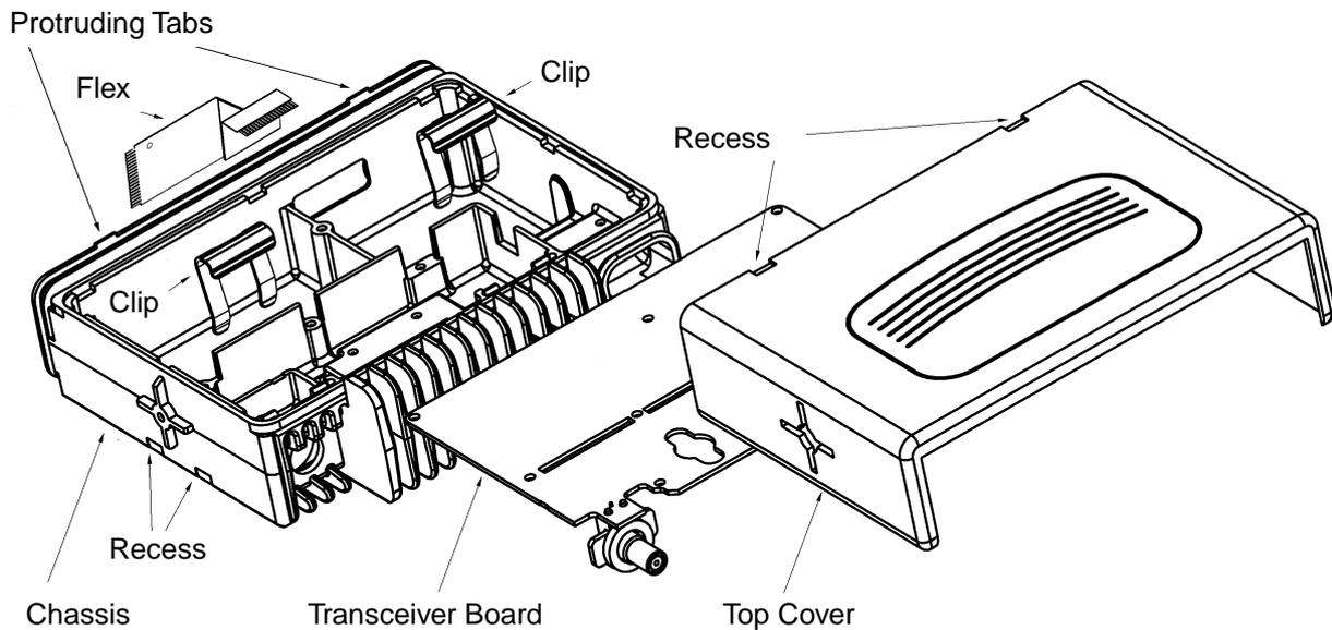
**Figure 2-3** Transceiver Board Removal.
