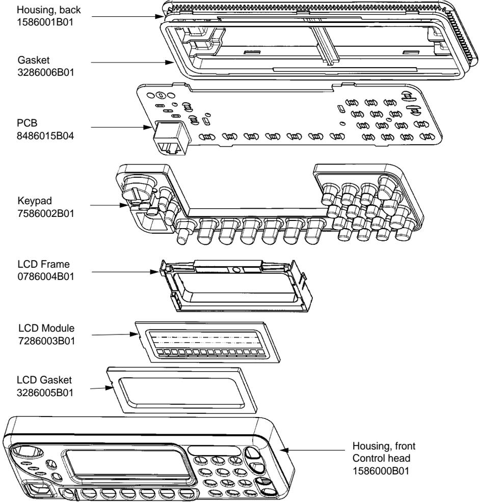
Figure 2-7 Control Head for Display/Keypad Radio Model.
