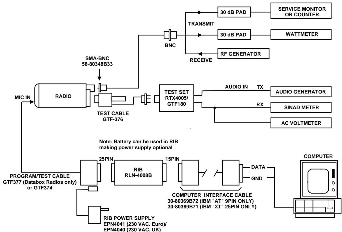
**Figure 4-1** Radio Alignment Test Setup
