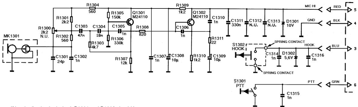
If level adjusting is desired, R1301 and R1302 should be taken out and be replaced by R1300 (p/n 1805500L04).
